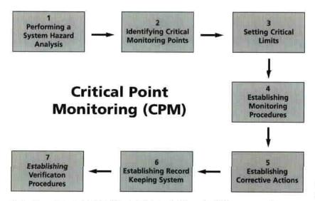
Using Hazard Analysis Critical Control Point principles, the CPM process outlines steps to systematically identify, monitor and control hazards associated with operating on-site systems to ensure safe system performance.
