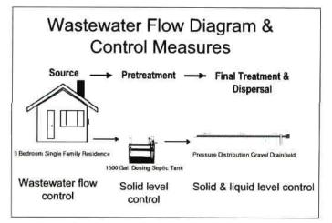
This diagram shows control measures at various points in a pressure distribution system flow path beginning at the source and continuing through treatment and dispersal into the environment. This tool helps determine where control measures are needed most.
